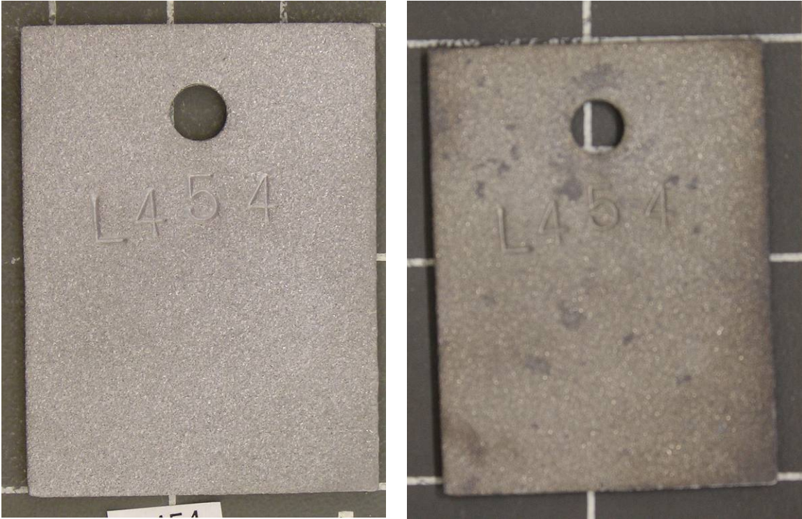
Figure 4-5 Images of lead coupon exposed to humid 3500 ppm CO 2 atmosphere. Left image shows coupon prior to experiments, right image shows coupon after six months exposure.
