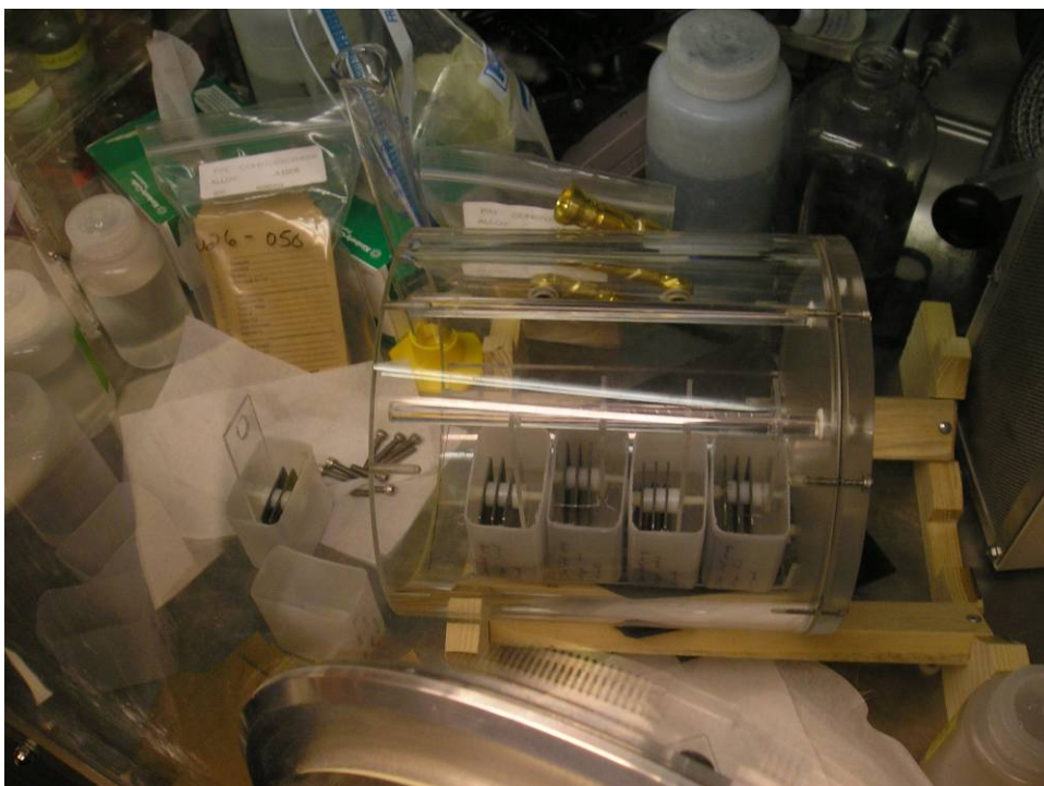
Figure 3-5 Partially loaded sample chamber inside the anoxic glove box. A second row of brine containers will be placed into the chamber and then the humid atmosphere replicates will be hung at the end of the chamber.
