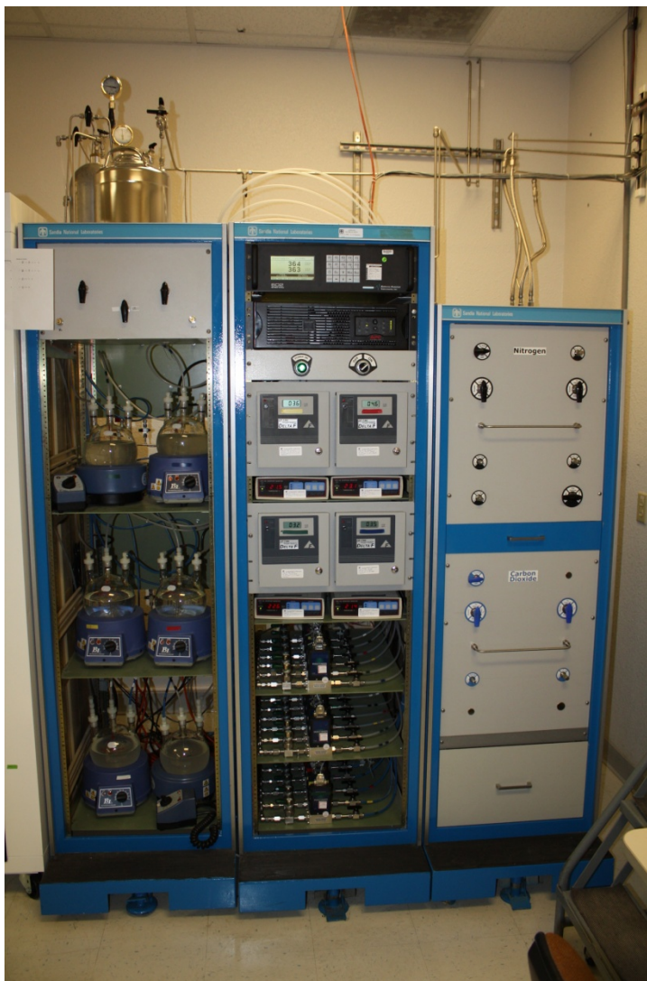
Figure 3-2 MFGCS Gas Distribution Panel (right) and Flow Controllers (bottom left).
