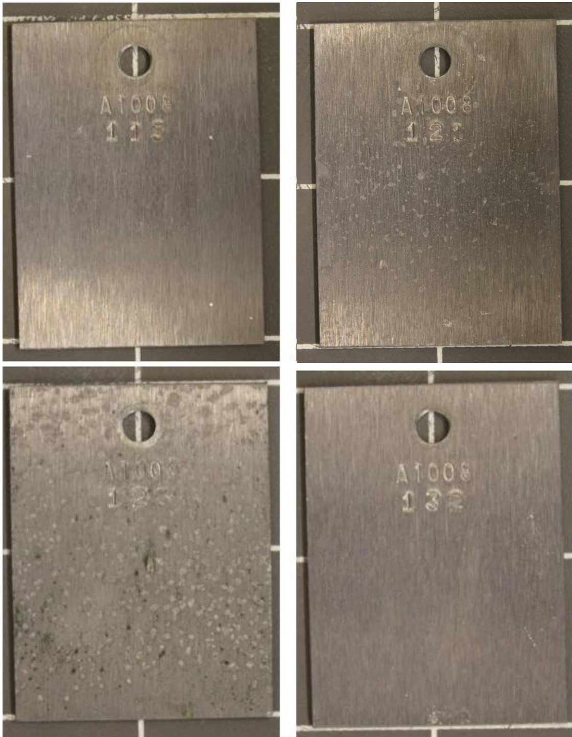
Figure 4-2 Photographs of fully immersed steel coupons after 6 months exposure in a 350 ppm CO 2 atmosphere. Coupon 115 (top left) submerged in GWB without organics. Coupon 121 (top right) submerged in GWB with organic ligands. Coupon 126 (bottom left) submerged in ERDA-6 without organics. Coupon 132 (bottom right) submerged in ERDA-6 with organic ligands.
